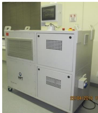
Figure 7: South African first 2.5kW Fuel Cell backup power system prototype. Source: (Sita, 2012)
