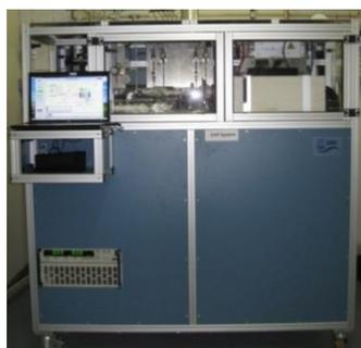
Figure 8: South African first 2kW HT-PEMFC combined heat & power unit for domestic applications. Source: (Sita, 2012)
