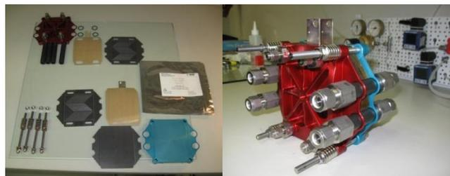
Figure 6: South African first HT-PEM fuel cell stack and bipolar plates. Source: (Sita, 2012)
