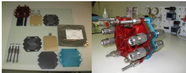
Figure 6: South African first HT-PEM fuel cell stack and bipolar plates. Source: (Sita, 2012)
