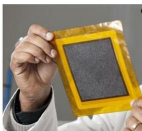
Figure 4: Figure First fuel cell electrodes (HT MEA). Source: (Sita, 2012)
